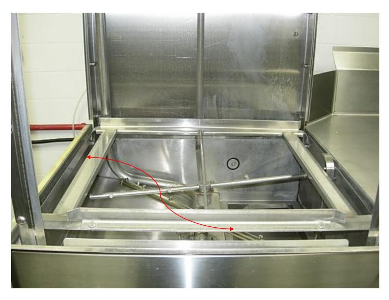
In order to convert machine from straight to corner application, you will need to relocate the tray track rail from straight to corner position (see red line on the photo) and then mount it on the tray track using the same bolts, washers and lock nuts used for straight application.
