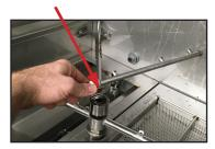
5. Verify the nozzles and arms are free from obstruction. If clogged, remove endcaps, clean nozzles with a brush, and flush with fresh water.
