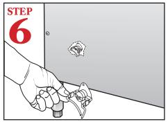
After filling dishwasher for the first time, (CAUTION: turn power supply off) reconnect the factory unplugged wire to booster high-limit switch located behind front panel.
